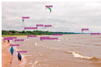
Fig.1 Object detection results recognized by one of famous algorithms, YOLOv3. The algorithm can detect small objects in the picture.
